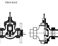
Style MA & MAS Single Seated Fully Balanced Direct Acting only SS Trim MA Sizes 3/4" - 1-1/2" Union Ends Bronze Body MA Size 2" Flanged Bronze or C.I. Body MAS Sizes 1" - 2" Flanged Steel Body MAS Sizes 3/4" - 1-1/2" Threaded Ends Steel Body
